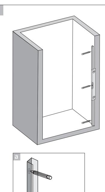
a Position and level the wall channels. Mark the fastening holes.
