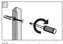
d Fasten the wall channel with ST4\*30 screws.
