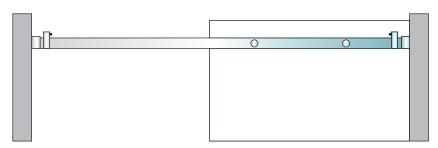
Attach rail to wall brackets by sliding wall bracket outer sleeves over the wall blocks and secure with grub screws.
