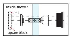
Attach Fixed Panel-Rail Connector to connect rail to fixed panel.
