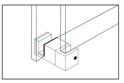
Hang door on the rail while fitting bottom edge into the floor guide and adjust wheel cam until level.
