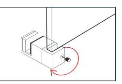
Ensure the floor guide is set to suit your desired composition (left or right). Then Proceed to use the grub screw to secure the guide to the bottom leading corner of the fixed panel.
