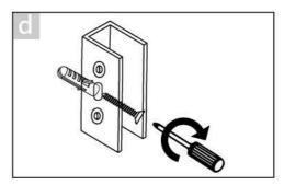
Fasten the wall brackets with ST4\*30 screws.
