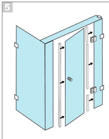
Fix hinge panel hinges to door panel, ensuring gaskets are fitted to each side of the glass when fitting hinges.
