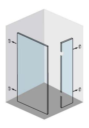
Insert hinge panel and return panel into wall brackets Fasten fixed panel & wall brackets.
