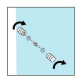
Cut 1 x side water seal into 3 parts to fit on the hinge panel. Fit 1 x side water seal on door panel.
