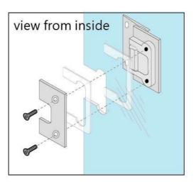
Attach Glass to Glass hinges to recesses in hinge panel ensuring allen head screws are facing the inside of the shower.
