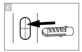
If no studs are behind the wall covering, use wall plugs when fastening the wall brackets.
