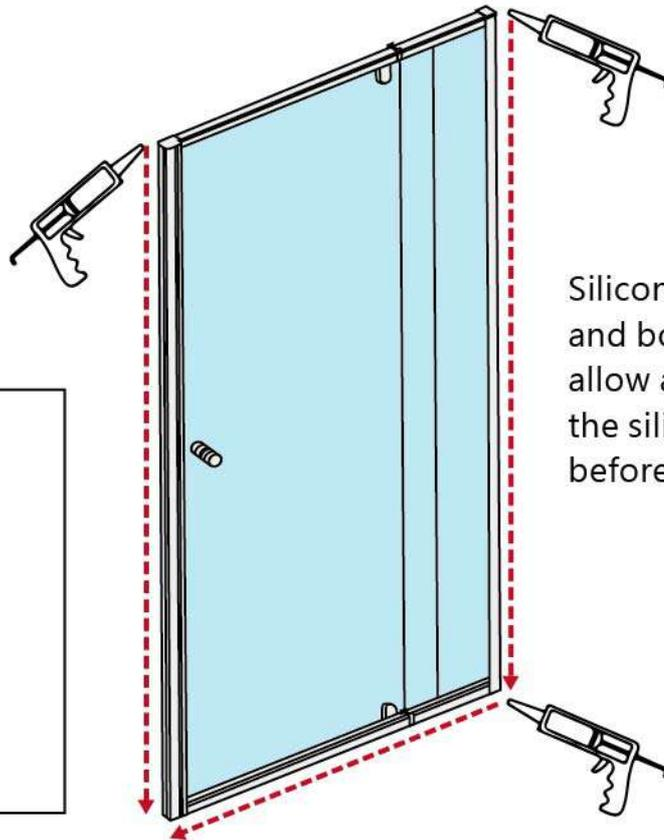
Silicone along wall channel and bottom track. Please allow at least 24 hours for the silicone to fully cure before using the shower.
